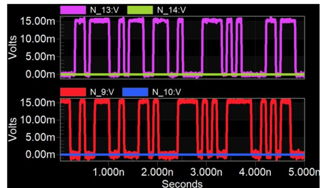
Fig. 2 Plot showing the In-phase component  $[I(t)]$  (N\_13 & N\_9 signal) and Quadrature component  $[Q(t)]$  (N\_14 & N\_10 signal) of two different BPSK frequency channels.
