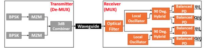
Fig 1. Block diagram of BPSK coherent detection demodulator.
