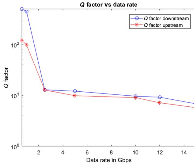
Fig. 7 Q-factor versus data rate per user.
