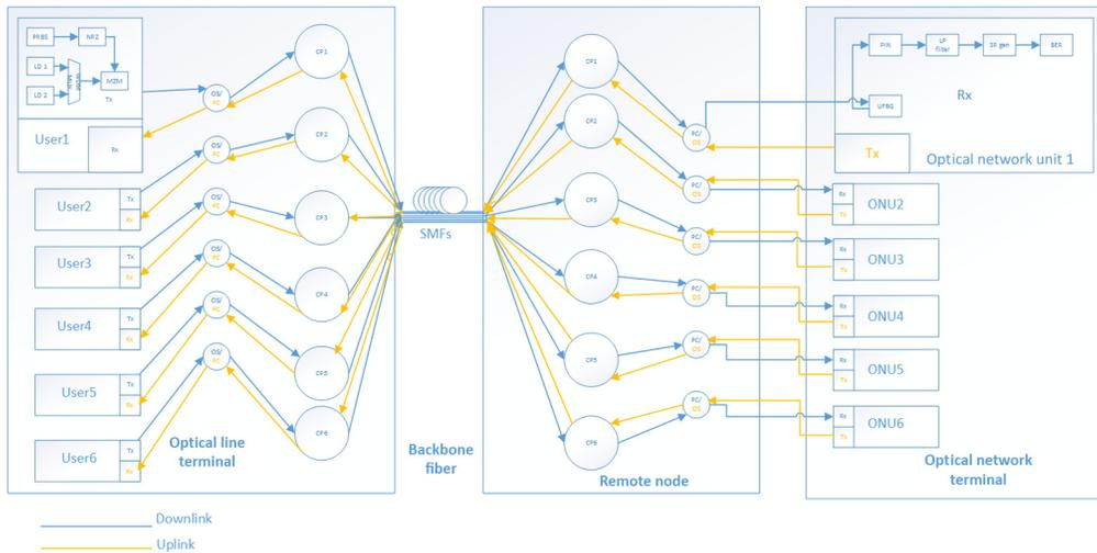
Fig. 1 Proposed system architecture of 2D-MD code-based OCDMA PON.
