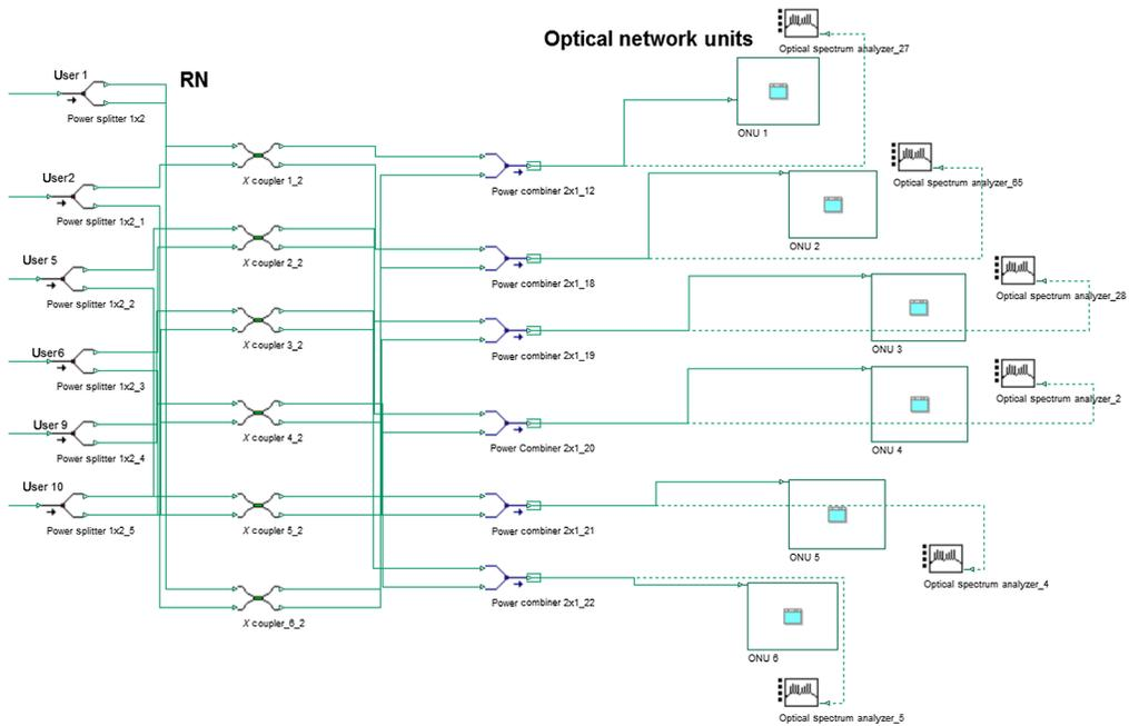
Fig. 3 RN design for 2D-MD code-based OCDMA PON.
