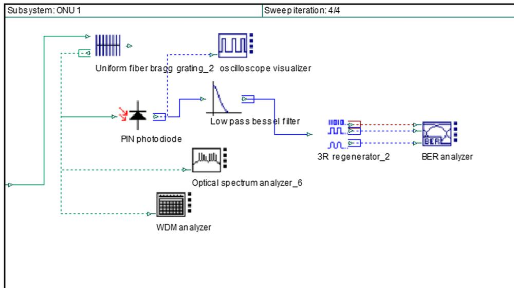
Fig. 4 Receiver design for 2D-MD code-based OCDMA PON.
