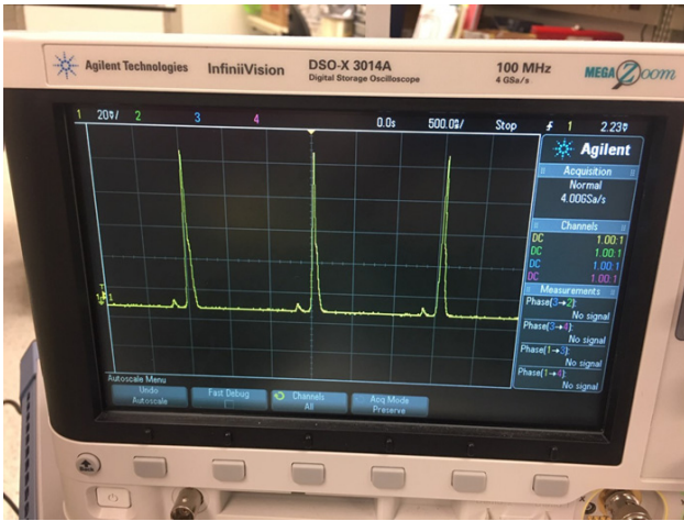
Figure 3: Active mode-locked laser output pulse train at 0.67 MHz repetition rate.
