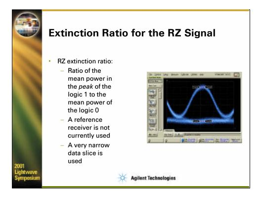
The NRZ measurement process does not apply to the RZ signal. First of all, due to the much shorter pulse duration of the RZ '1', the "mean" power in a logic 1 will have a value that is somewhere close to half the amplitude of the signal. Currently, no standard reference receiver is used in the measurement thus no integration function is achieved.
