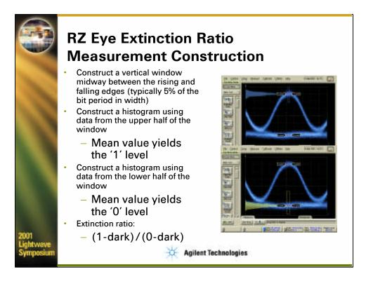
The diagrams show the histograms from which the critical data is obtained. (These are shown for explanatory reasons. In actual measurements the histograms are not visible on the screen unless set up manually). For the highest measurements accuracy, the dark level must be determined (through a calibration) and removed from the measurement result.
