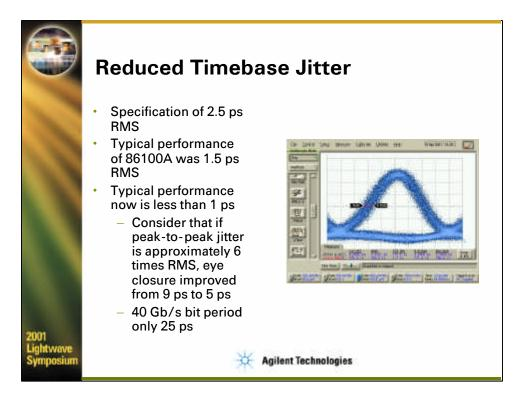
The jitter of the 86100 is specified at 2.5 ps rms. This would yield a peak-to-peak value of approximately 15 ps. Considering that the full bit period of a 40 Gb/s signal is only 25 ps, eye closure due to instrument jitter would be significant.
