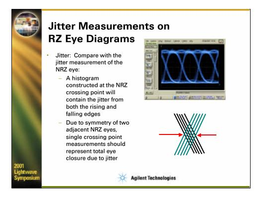
The procedure for jitter measurements of the RZ eye must also deviate from the NRZ case.
