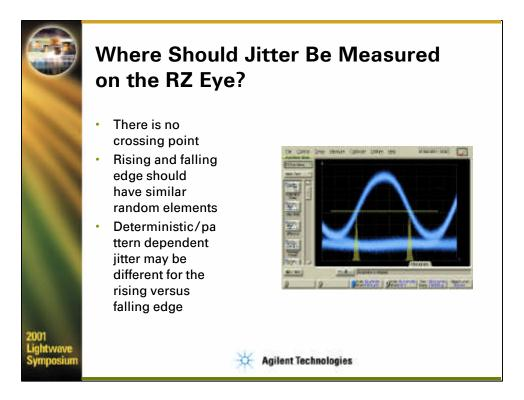
The jitter measurement for the RZ measurement cannot rely on the symmetry of the eye to determine the eye closure due to jitter with a single measurement. Once again, because there are no crossing points.
