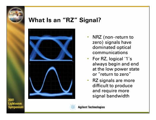
The RZ signal transmission of a logic '1' will always begin at zero and end at zero. The lower of the two diagrams shown is of the RZ eye diagram. It is a composition of several transmitted 1's and 0's overlaid on top of each other in a single display. Note how all '1' pulses, whether they are preceded by and followed by a 1 or a 0, start and end at the low power state.
