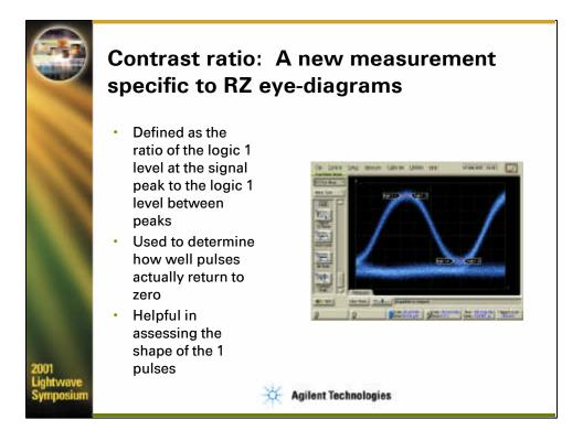
Contrast ratio is a new measurement unique to the RZ signal. Ideally a logic '1' pulse should begin at a zero power level, rise up to the peak power of the signal, and then return to zero power. In this ideal case, the ratio of the peak of the '1' pulse to the '1' level at its lowest power would be infinite.
