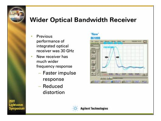
The Agilent 86109B integrated optical receiver has an optical channel with over 40 GHz of bandwidth and an electrical channel with 50 GHz of bandwidth. (The previous generation of receivers had a bandwidth of 30 GHz using the 86109A, while the 86106A had 20+ GHz bandwidth but with significant pulse distortion).
