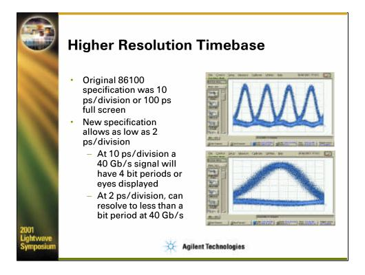
The last recent improvement is in timebase resolution. The original 86100 mainframe minimum timebase setting was 10 ps/division. Thus the full screen would cover 100 ps. For a 40 Gb/s signal, four full eye diagrams will be displayed. Since two adjacent eye diagrams contain virtually the same information, 75% of the display provides no useful information.
