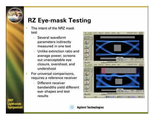
Eye mask testing can also be implemented for the RZ signal. Recall that the intent of the NRZ mask test is to quantify the shape of the eye diagram. It is important to note that the shape of the eye can be dramatically affected by the bandwidth and frequency response of the test system.
