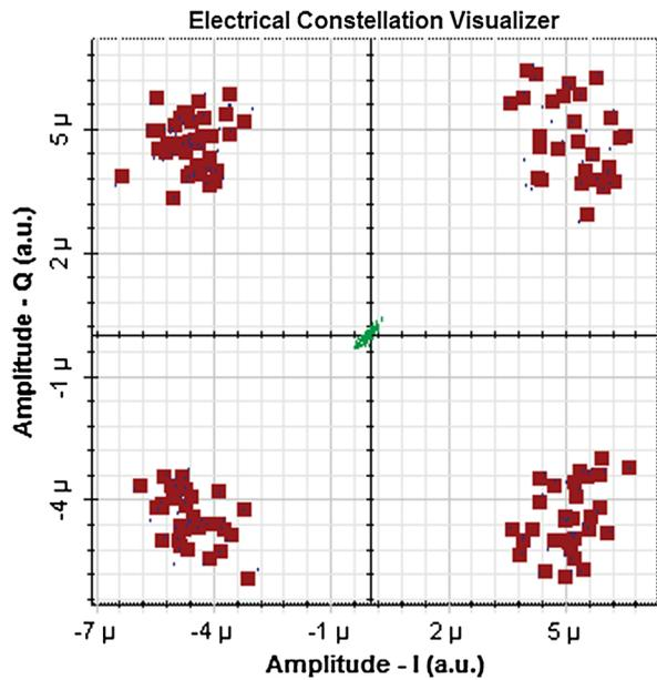
Fig. 7 Electrical constellation diagram.
