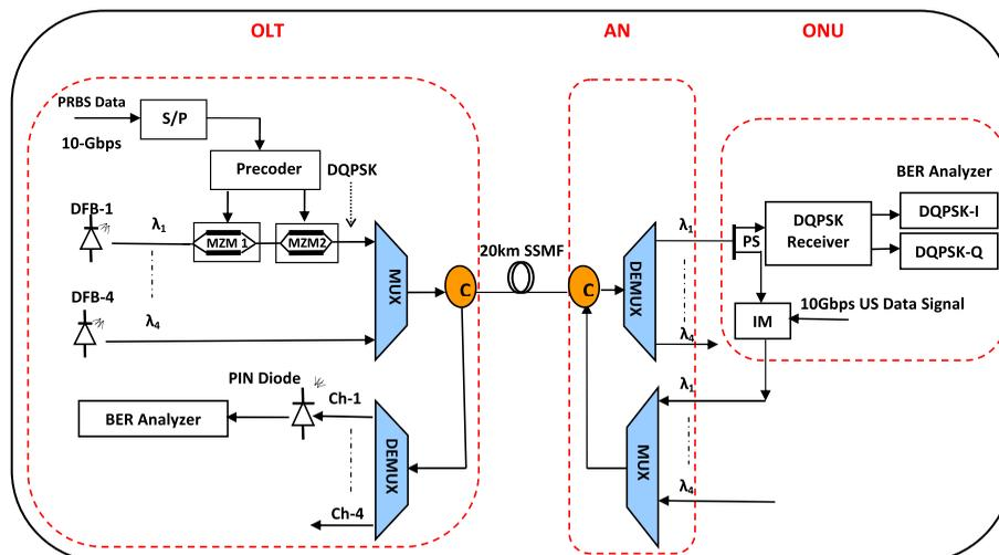
Fig. 1 Schematic diagram of single feeder full duplex WDM-PON system.
