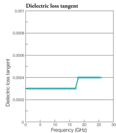
Measurement method: Triplate rail resonance method
