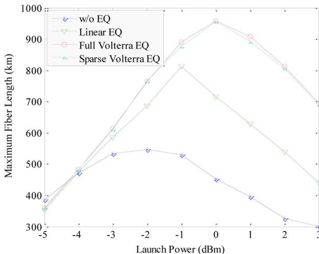
Fig. 6. 16-QAM CO-OFDM systems' maximum transmission distances at  $10^{-3}$  BER versus launch power.
