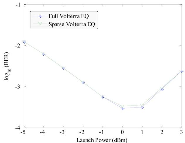
Fig. 4. BER of 16-QAM CO-OFDM systems with full or sparse Volterra equalizers as a function of launch power.
