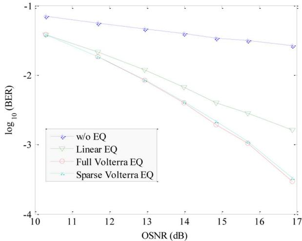
Fig. 5. BER of 16-QAM CO-OFDM systems w/o compensation and with linear/nonlinear equalization as a function of OSNR (fixed launch power).
