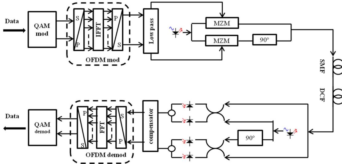
Fig. 1. Block diagram of CO-OFDM system.
