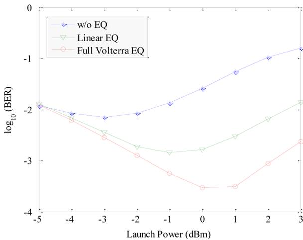
Fig. 3. BER of 16-QAM CO-OFDM systems w/o compensation and with linear/nonlinear compensation as a function of launch power.
