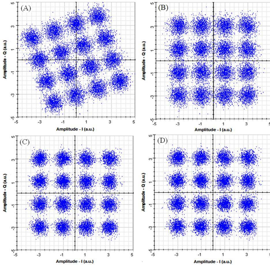
Fig. 2. Constellation of 16-QAM CO-OFDM system. (A) w/o equalizer, (B) with linear equalizer (C) with full Volterra equalizer (D) with sparse Volterra equalizer.
