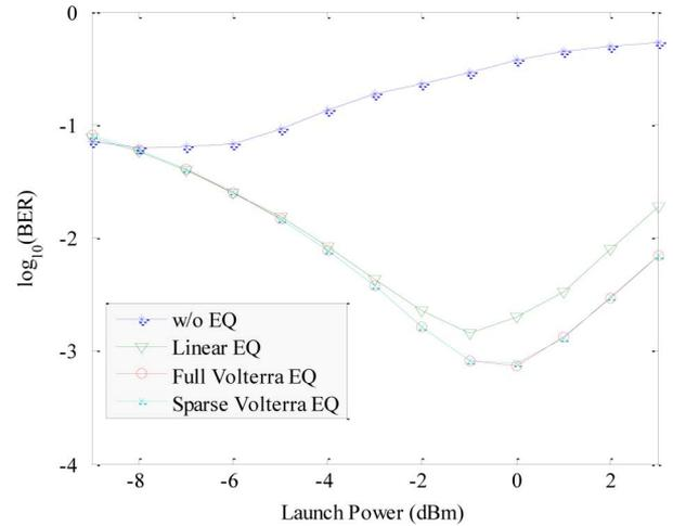
Fig. 7. BER of 5 channel WDM 16-QAM CO-OFDM systems w/o compensation and with linear/nonlinear compensation as a function of launch power.
