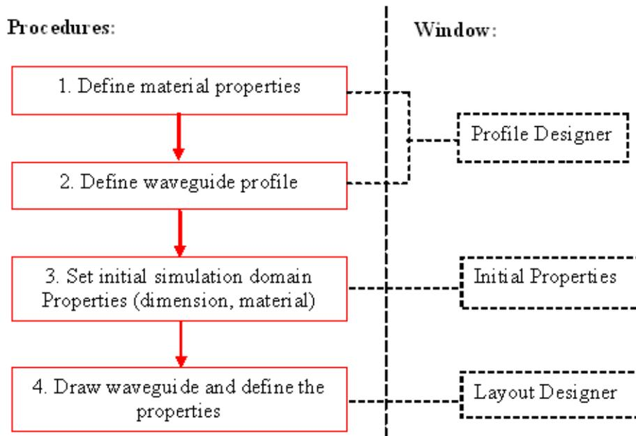
**Figure 1** Flow chart for building a Layout
