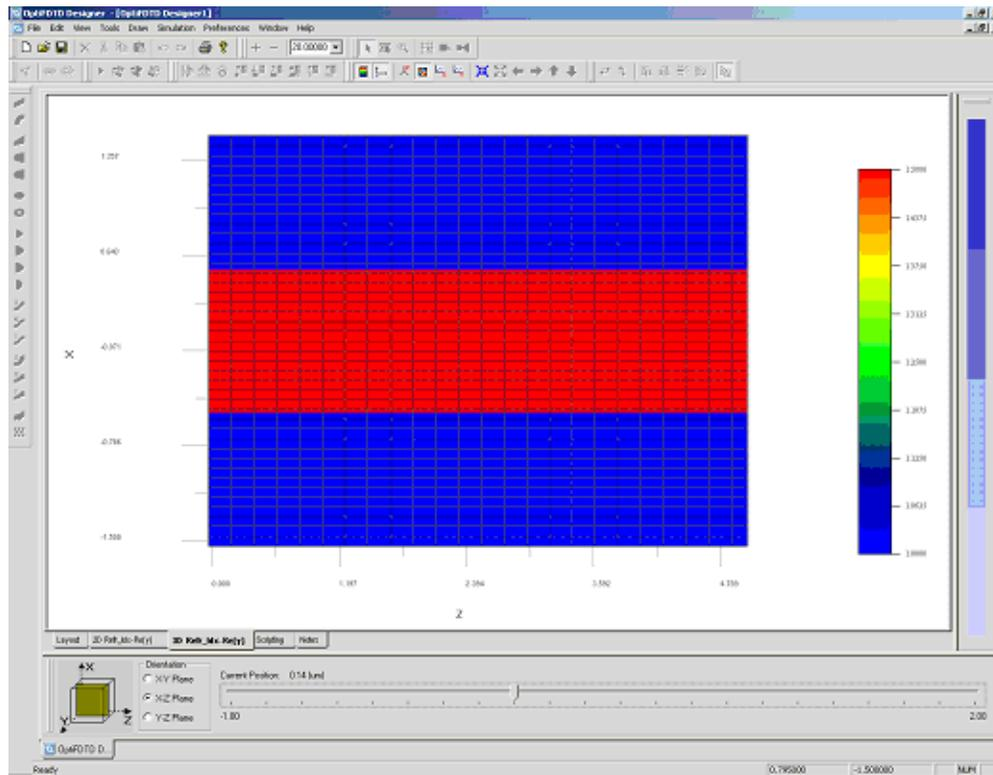
Figure 4 Refractive index in x-y orientation at z=0
