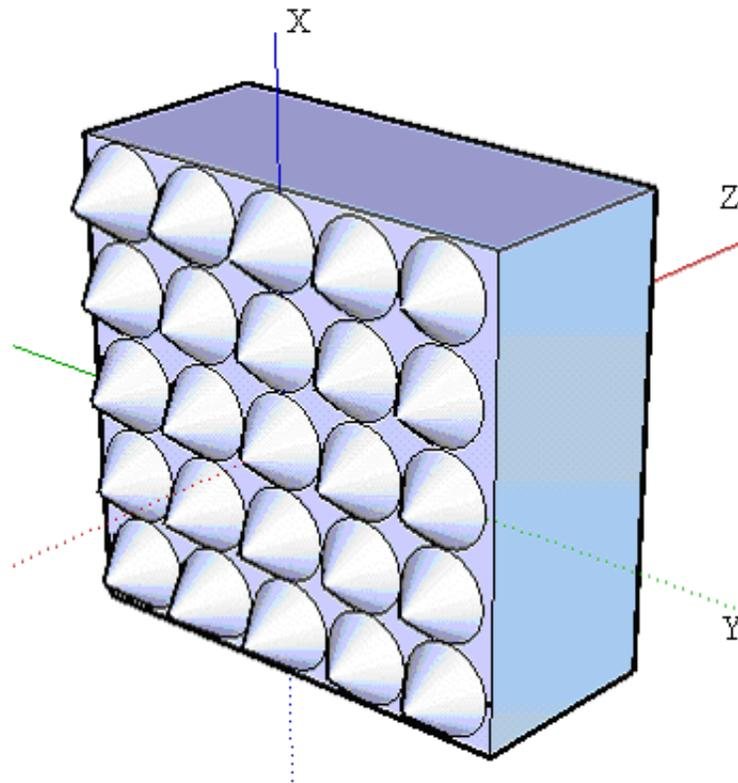
The layout represents a square of periodic cones with height (z-direction length) of  $1\mu\text{m}$  deposited on the flat substrate. The diameter of the cone's bottom is  $1\mu\text{m}$ , the
