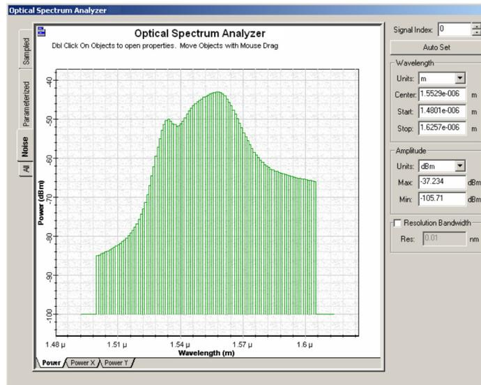
Noise Bins can be created whenever there is a source of optical noise, such as optical amplifiers. You define the initial resolution and bandwidth of the noise (see [Figure 46](#)).
