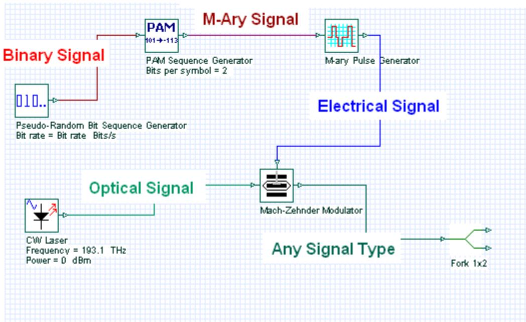
OptiSystem handles mixed signal formats in the Component Library for optical and electrical signals. It calculates the signals using different algorithms according to the desired simulation accuracy and efficiency.
