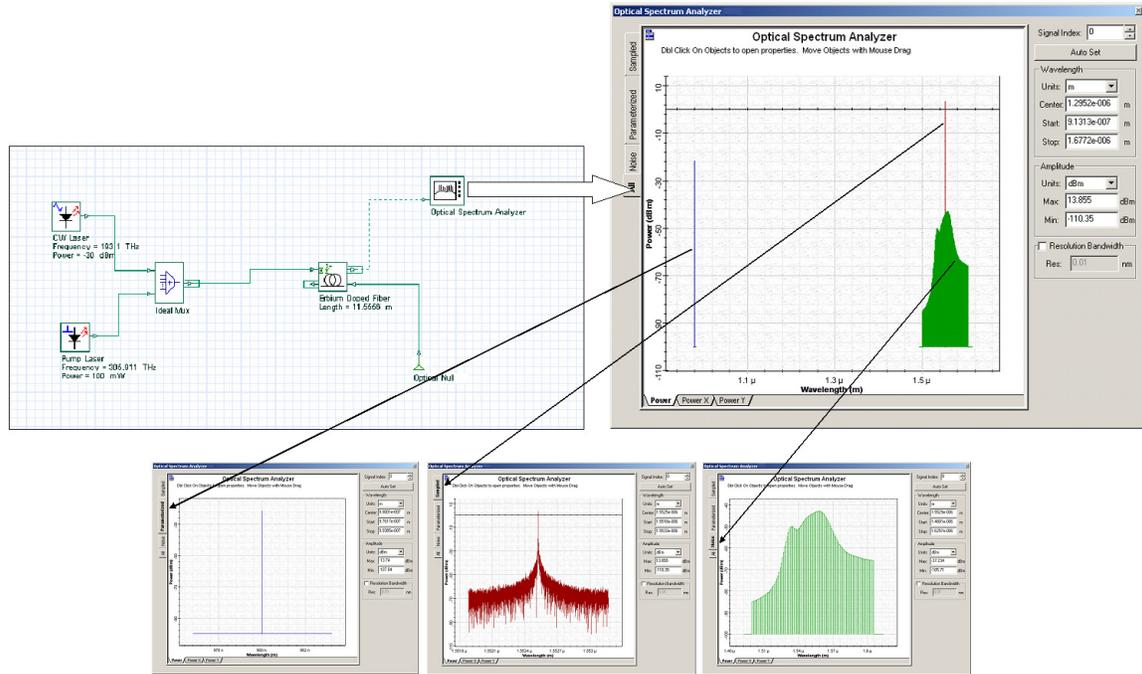
During transmission, the widths of the noise bins are adapted automatically to describe the filtering of the noise with a specified precision. The noise bins shrink in width as they propagate through the simulation in order to maintain the discretization accuracy (see [Figure 47](#)).
