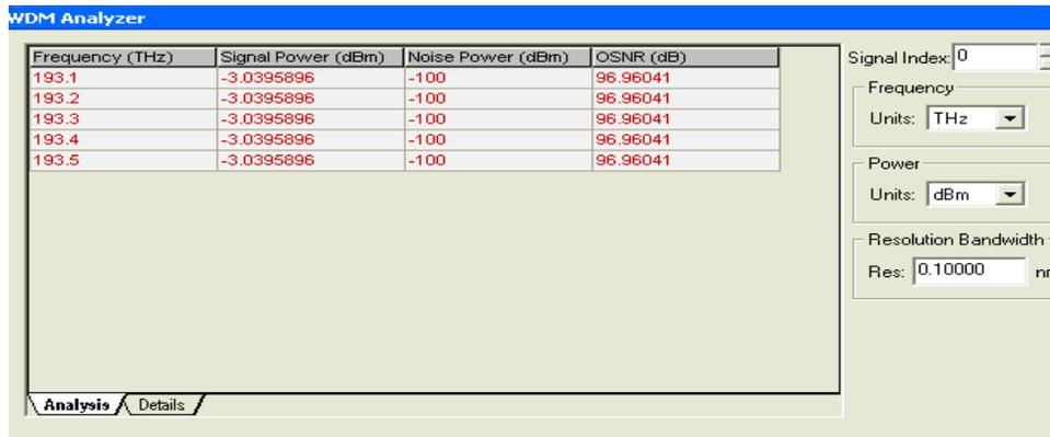
Fig.11 Properties of the WDM analyzer of the five channels
