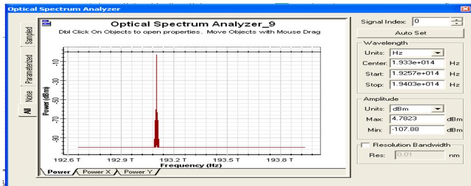
**Fig.10** The OSA of the reflected channel of the ideal dispersion compensation FBG for the first demultiplexer subsystems.
