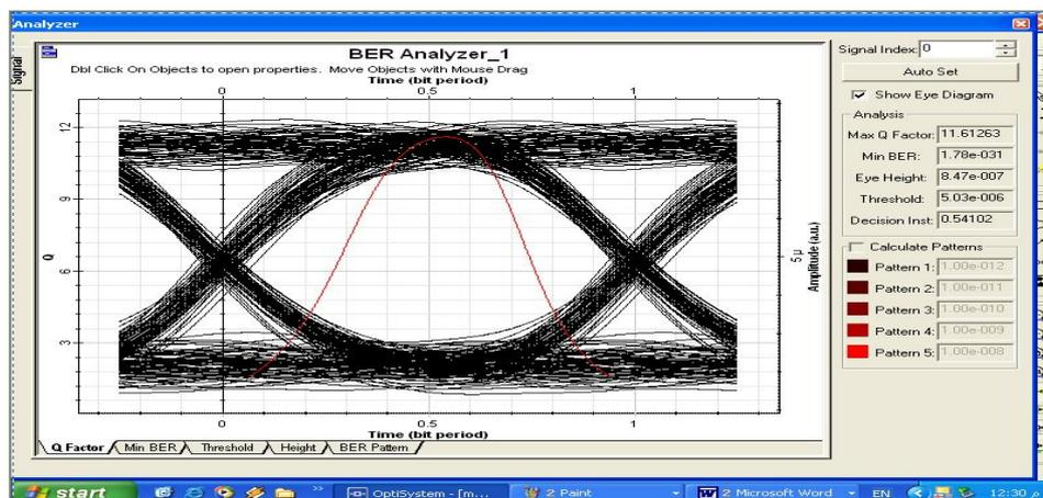
Fig.12 Q- Factor and BER of the first demultiplexed signal (BER-1)
