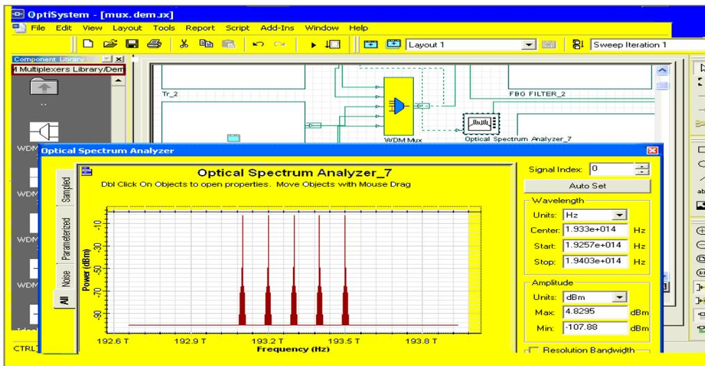
**Fig. 4 Optical spectrum analyzer of WDM multiplexer**
