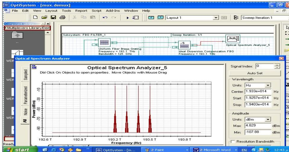
**Fig.9** The OSA of the transmitted channels of the ideal dispersion compensation FBG for the first demultiplexer subsystems.
