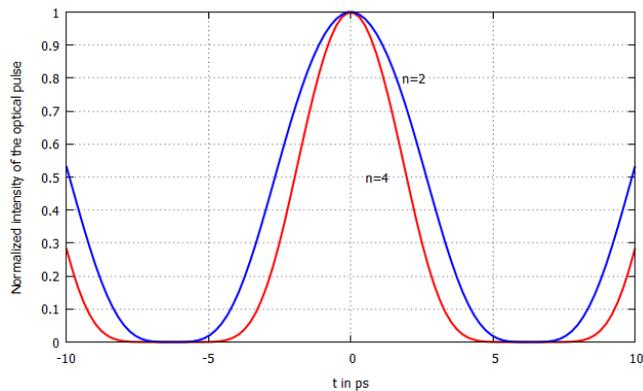
**Fig 3** Same as in Fig.1 showing a single pulse. “n” corresponds to the number of M-Z modulators.
