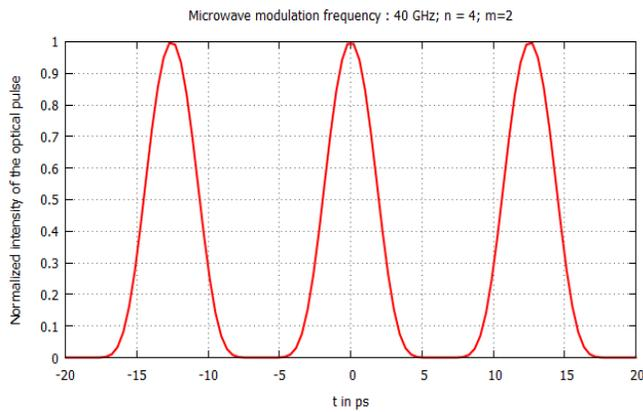
**Fig 2** Variation of the normalized intensity of the generated optical pulse with time
