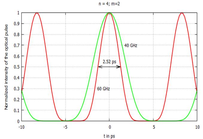
**Fig 4** Normalized intensity profile of the pulse using microwave modulation frequency as parameter
