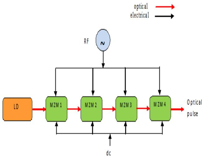
**Fig 1** A schematic circuit diagram of the proposed optical pulse generator. LD: laser diode; MZM: Mach Zehnder modulator ; RF: microwave modulating source ; dc: dc bias
