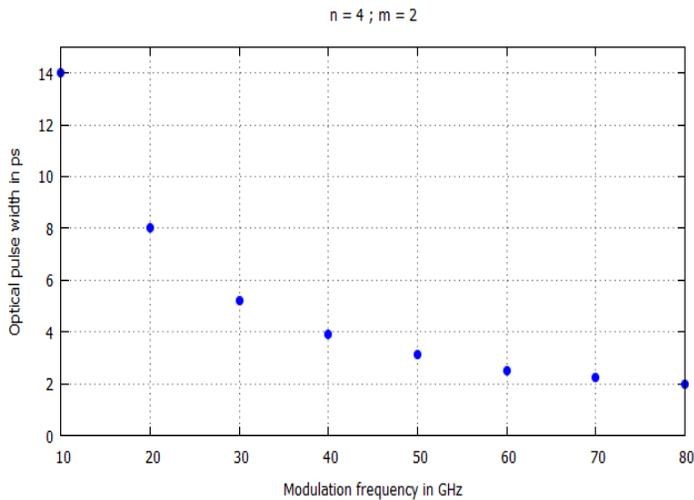
**Fig 5** Variation of generated optical pulse width with applied modulation frequency.
