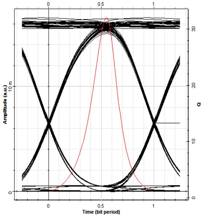
Fig. 8. Eye diagram of downlink channel of BS 1
