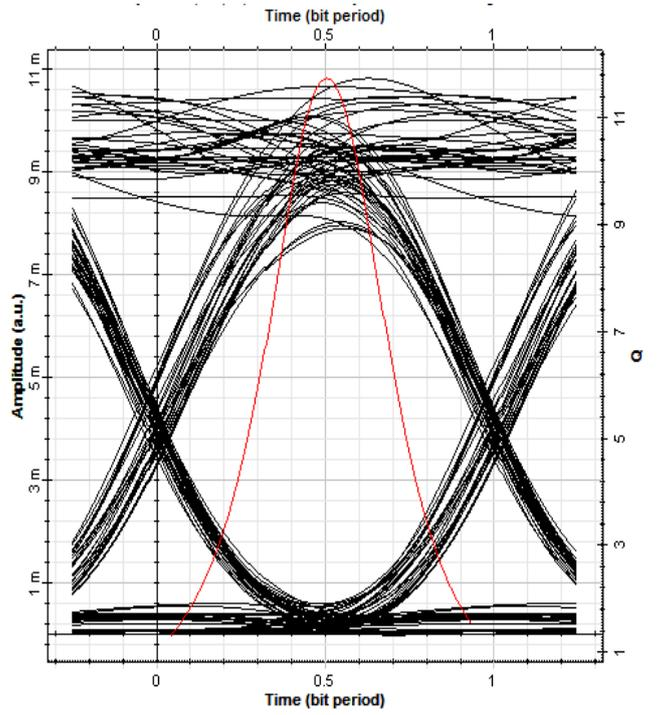
Fig. 10. Eye diagram of uplink channel of BS 1
