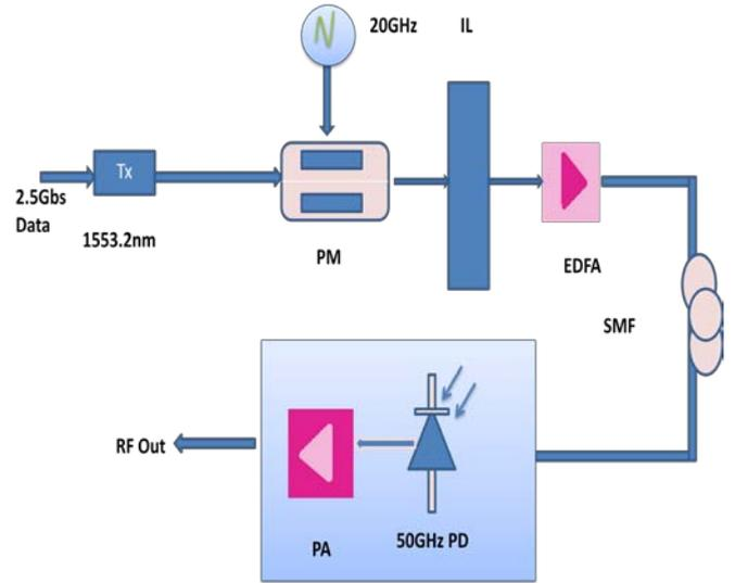
Fig. 1. Experimental model of single channel RoF system
