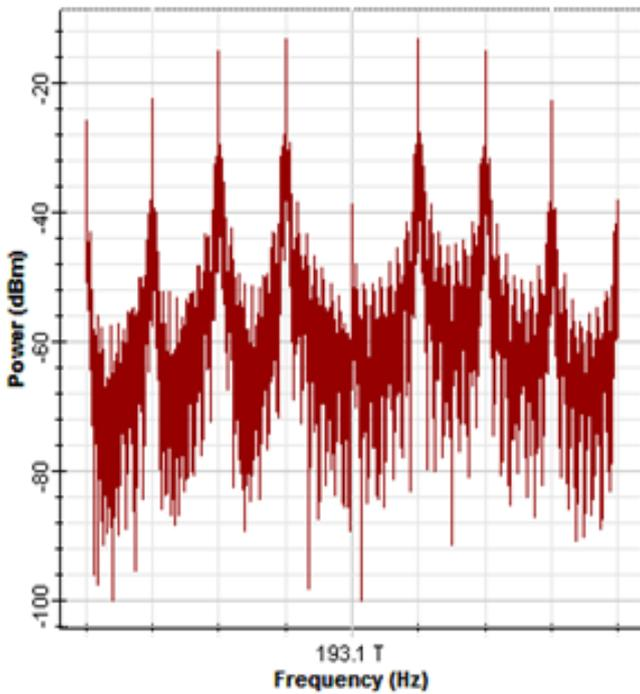
Fig. 4. Carrier suppressed spectra of channel 1
