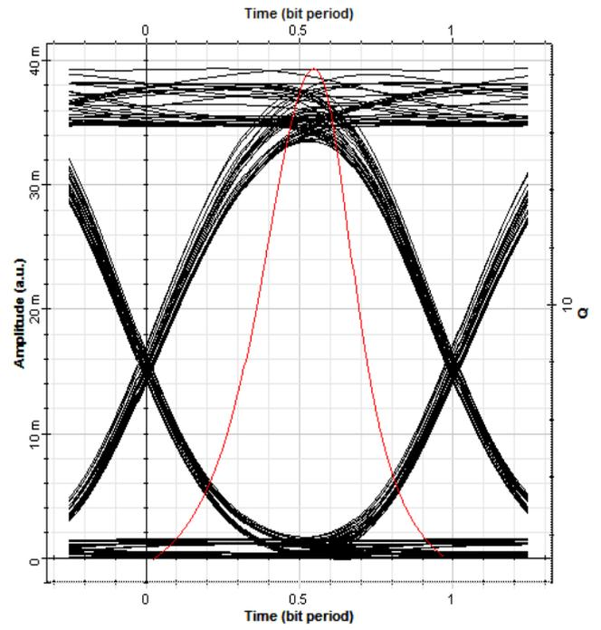
Fig. 9. Eye diagram of downlink channel of BS 2
